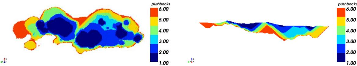
Figure 3: Plant view (left) and section view (right) of pushback selection from McLaughlin mine.
