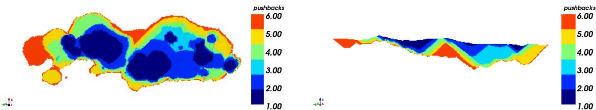
Figure 3: Plant view (left) and section view (right) of pushback selection from McLaughlin mine.
