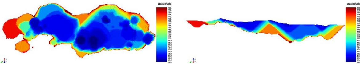
Figure 2: Plant view (left) and section view (right) of nested pits map, McLaughlin deposit.
