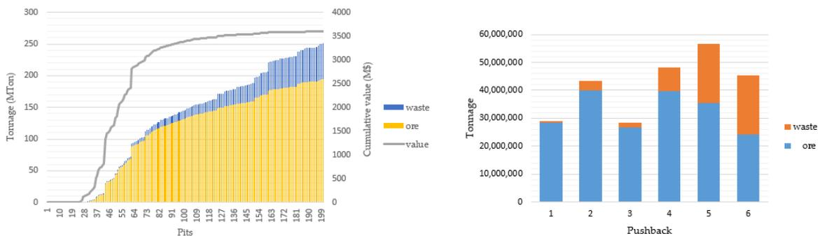
Figure 4: Pit by pit graph (left) for 200 nested pits. Tonnage graph (right) of pushback selection from McLaughlin mine.
