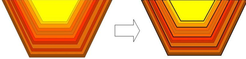
**Figure 1:** Nested pits generated by a parameterization of the metal price. Some of these pits are selected as pushbacks.
